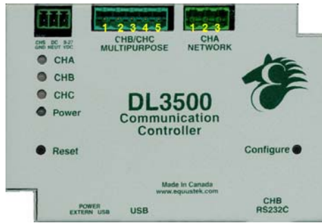
Pin Numbering for the DL3500
