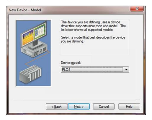
In device ID enter the node address number of the Processor you are trying to communicate with, in this example here, the PLC5 node address number is 21 Octal, from the drop menu please make sure to select the right format for the device ID (Node address number), All Allen Bradley SLCs and PLCs on DH+ are all in Octal. So either enter 21 and select Octal, or convert the node number to Decimal enter 17 and select Decimal.
