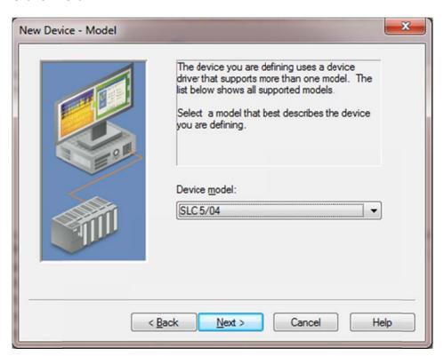
In device ID enter the node address number of the Processor you are trying to communicate with, in this example here, SLC504 node address number is 03 Octal, from the drop menu please make sure to select the right format for the device ID (Node address number), All Allen Bradley SLCs and PLCs on DH+ are all in Octal. So either enter the octal ID and select Octal, or convert the node number to Decimal and select Decimal, here 03 octal is equal 03 decimal, but it matters when ID is bigger than 07.
