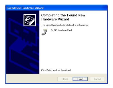
In the Device manager, check the comport number for the DLCPI and remember it to use in configuring the Allen Bradley DF1 driver.
